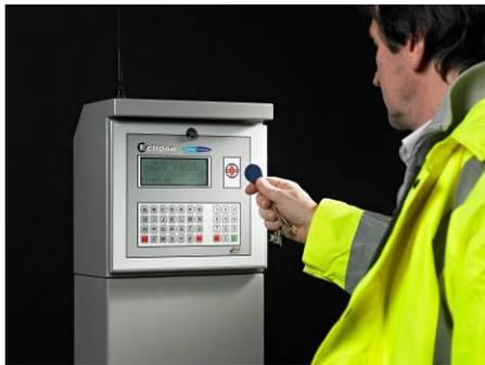
The Fuel Island Controller is the user interface for the pumps on site. Before fuelling the user must ID the vehicle to be fuelled (eg using a tag or card) and then may be prompted for other information such as mileage or registration number. The fuel island is configured to match the site it is installed on so that it can make decisions on what pumps to offer, or what ID methods to accept. This set up is only required once, when the system is installed.
